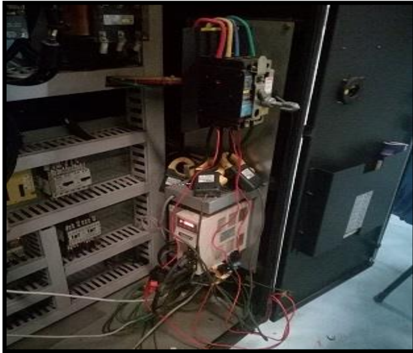
Fig.6 power analyser setup
