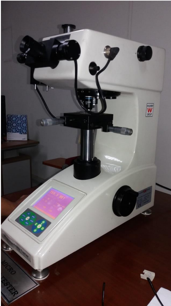
Figure 15: Micro Vicker hardness machine
