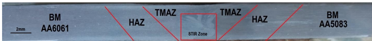
Figure 36: Weld cross-section with distant zones
