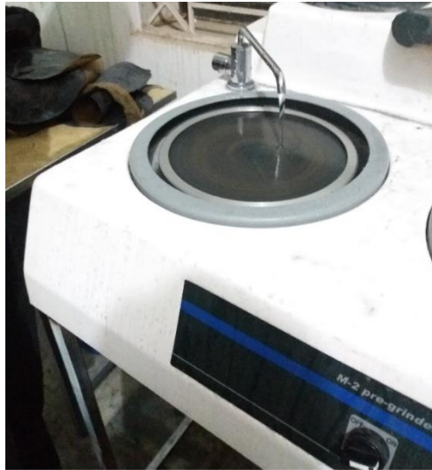
Figure 19: Grinding machine used for samples
