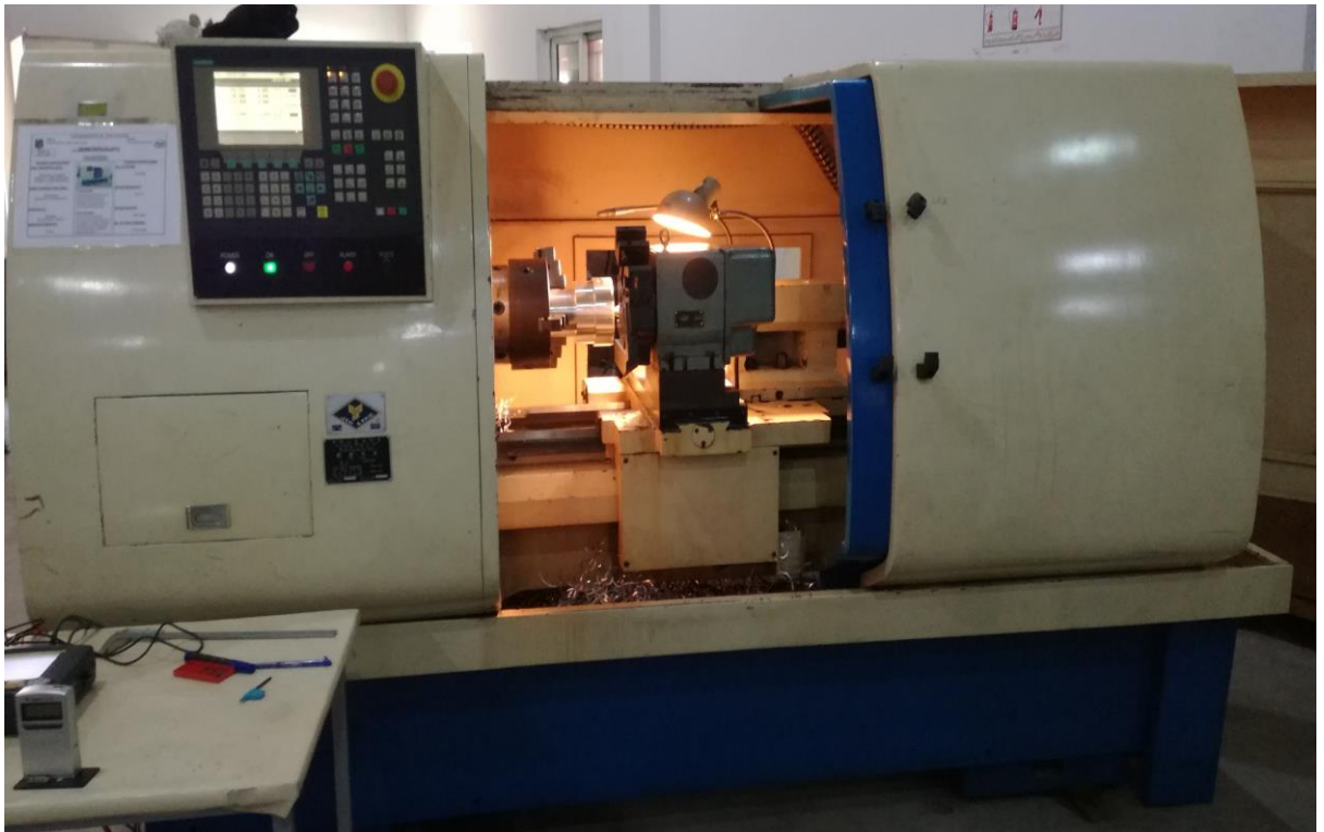
Figure 3: Turning Centre (Model: CK 6150) at LESC Gujranwala
