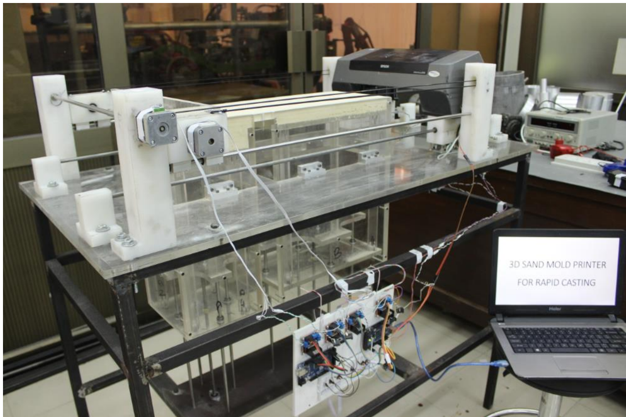
Figure 27 Developed 3D Sand Mold Printer Setup
