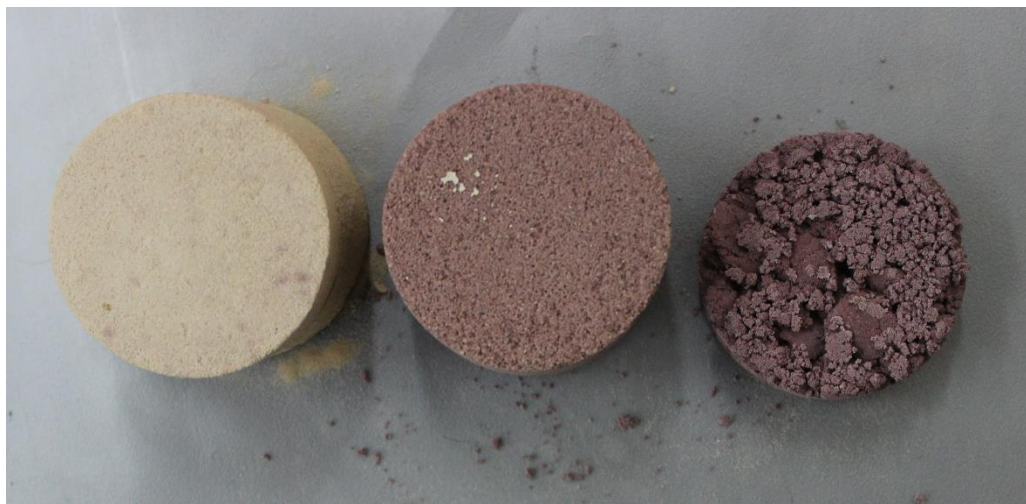
Figure 14 Initial Test Specimens Using Traditional Ramming Method
