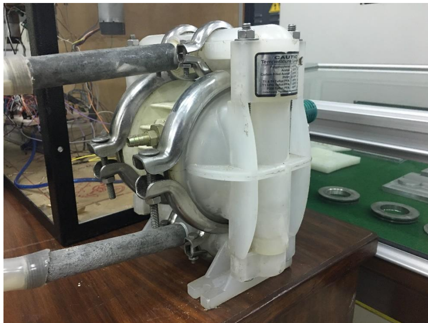
Figure 28: An air operated dual diaphragm (AODD) pump
