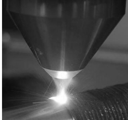
Figure 10: Deposition of Metal Coating upon a pipe using Co-axial Laser Cladding process
