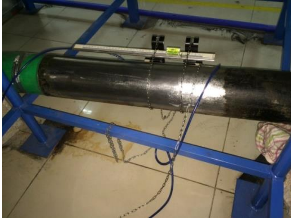
Figure 3.1.2: Transducers installed on discharge pipe
