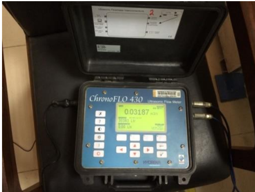
Figure 3.1.1: Ultrasonic Flow Meter Display
