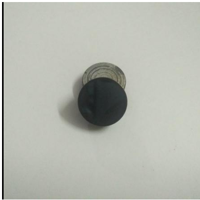
Sample Coated in Photoresist
