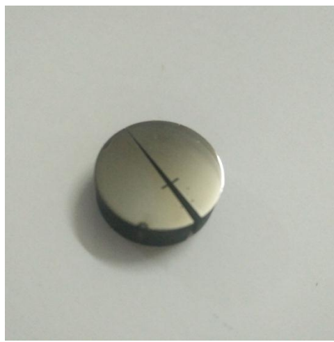
Sample Cross Sectioned for Kerf Angle
