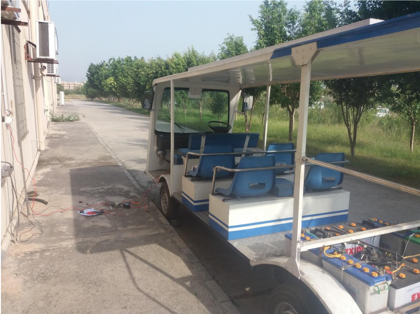
Figure 17 Electric Vehicle (Battery Bank)
