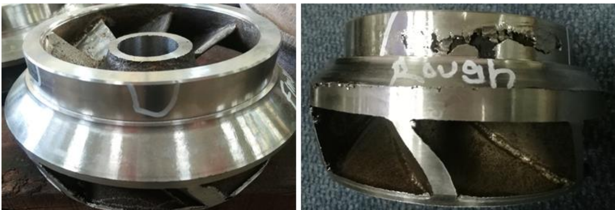
Figure 6. 4 Confirmation test for Shrinkage porosity
