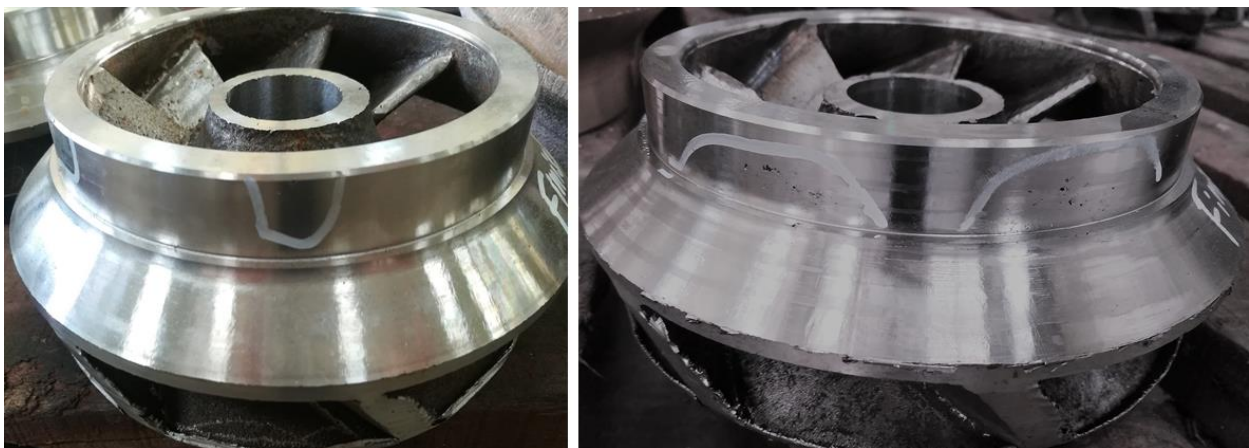
Figure 6. 6 Confirmation test for Blow hole
