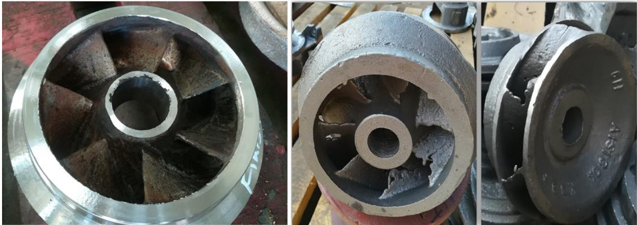
Figure 6. 5 Confirmation test for Misrun
