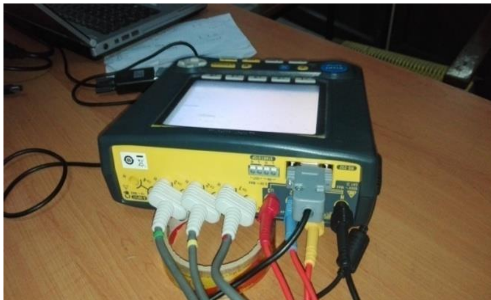
Figure 5 Yokogawa Power Analyzer CW-240
