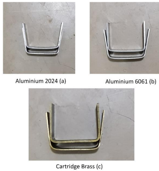
Figure 2.14: workpieces after U-Bend
