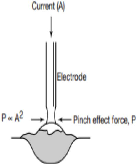
Fig.2 short circuit Heat Transfer
