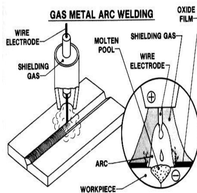
Fig.1 Gas Metal Arc Welding Process
