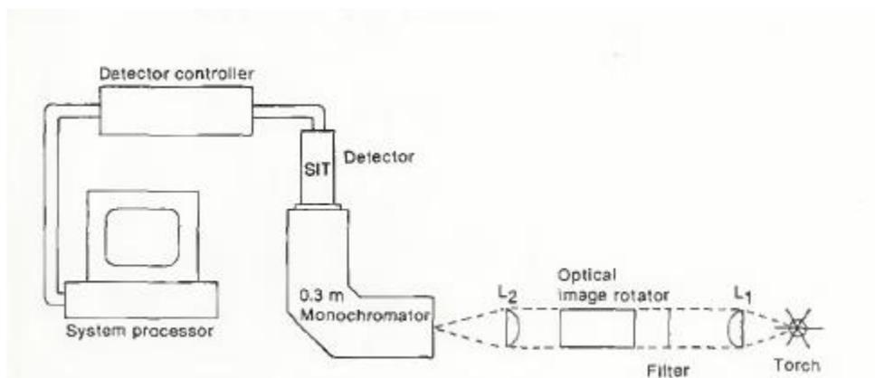
Fig. 6 Experimental Layout of the Apparatus used for optical image Spectroscopy.
