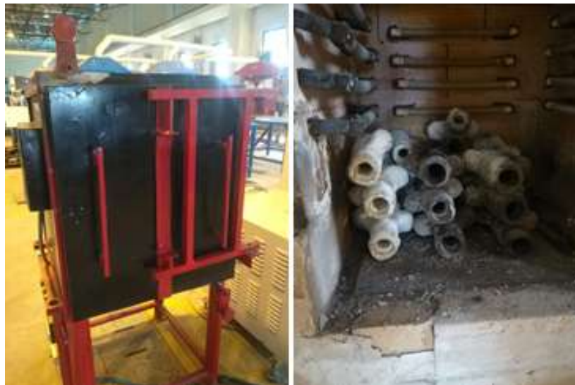
Figure 2.16: Burnout oven/ Heating furnace
