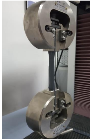
Figure 18 Tensile Test using UTM
