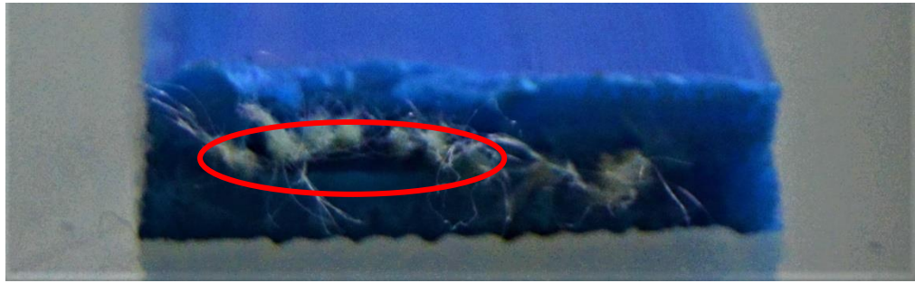
Figure 44 Cross-sectional view of Flexural sample
