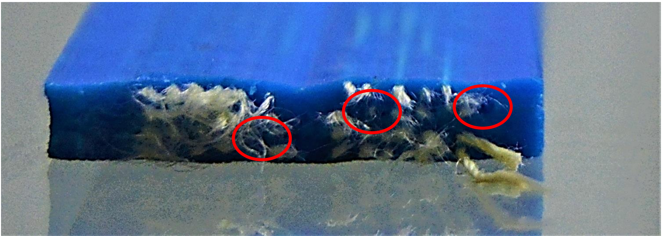
Figure 46 Cross-sectional view of Tensile sample and void formation
