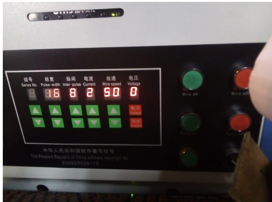
Figure 3.2: Parameters of EDM for creating notches
