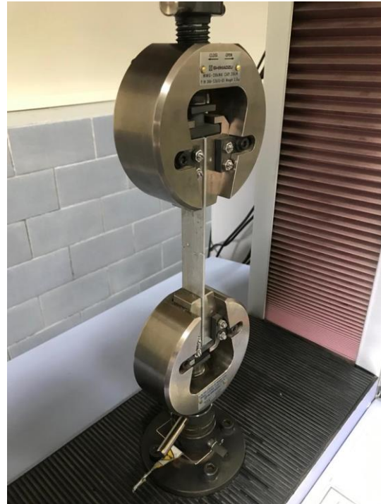
Figure 3.8: Side view of sample in hydraulic jaws
