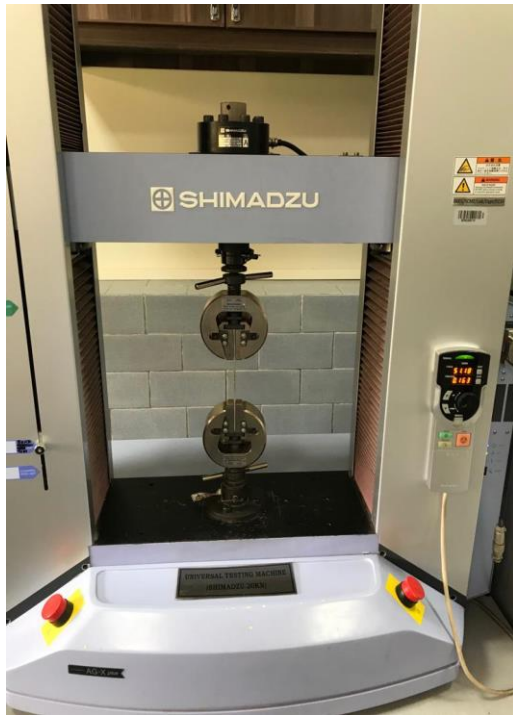
Figure 3.7: Hydraulic jaws holding sample
