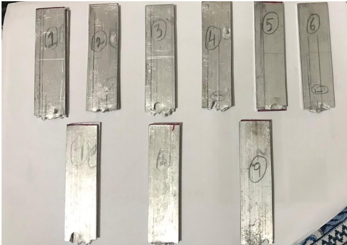
Figure 4.10: Breaking of samples after tensile testing
