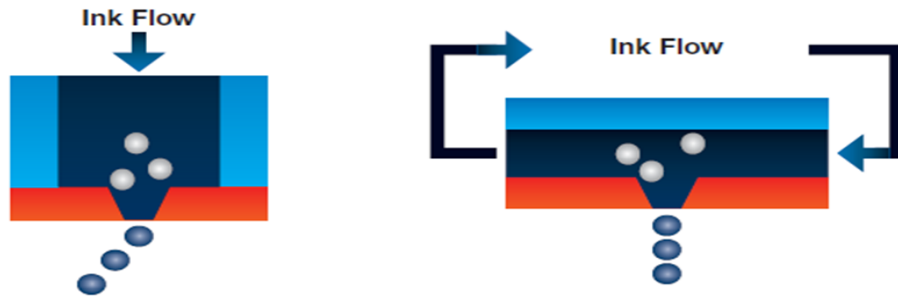
Figure 28 End Shooter VS Xaar's Hybrid Side Shooter Technology
