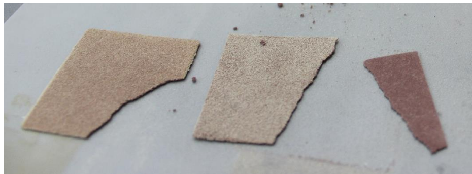
Figure 16 Initial Test Specimens Using Manual Layer by Layer Deposition
