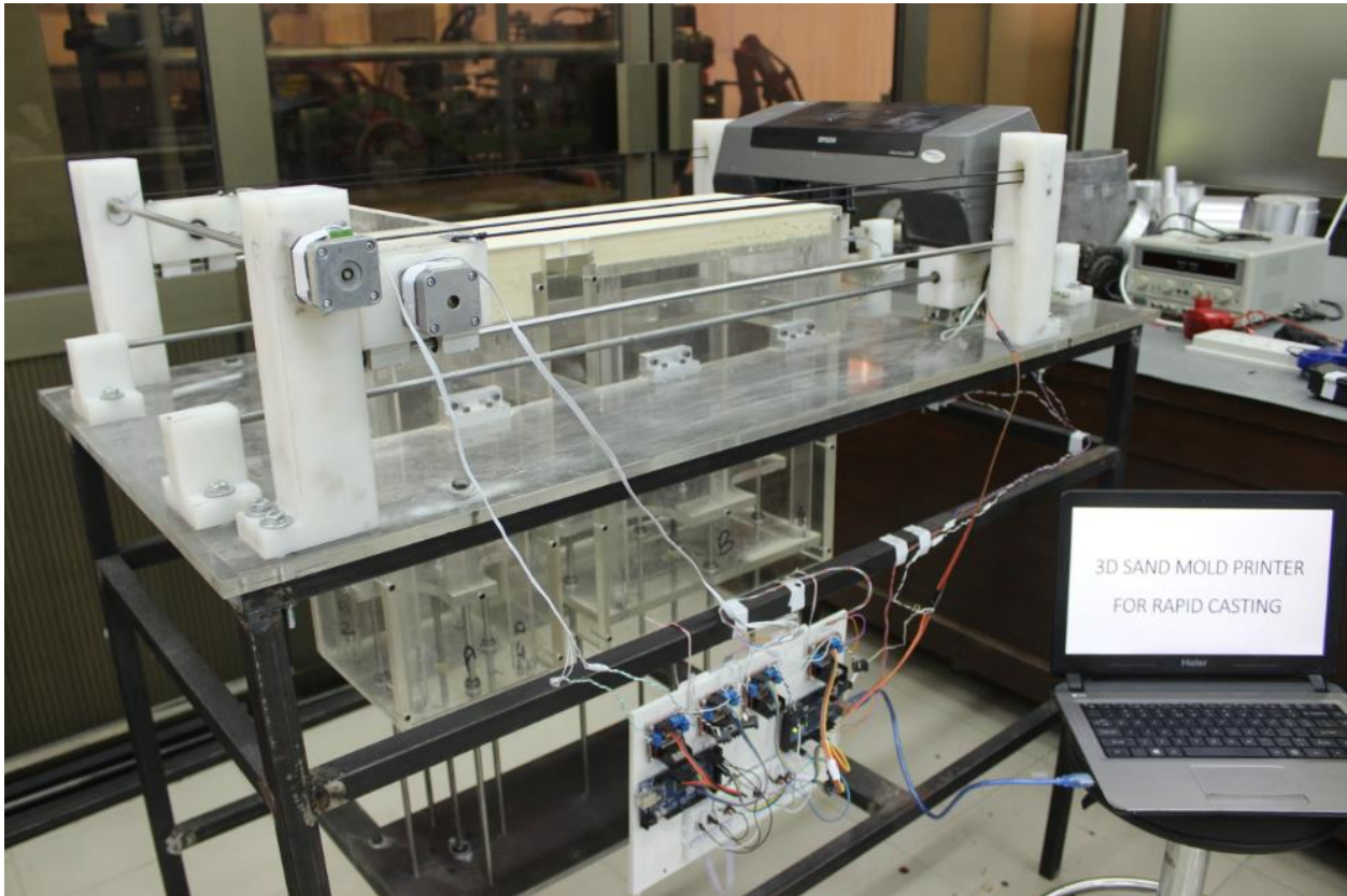
Figure 27 Developed 3D Sand Mold Printer Setup
