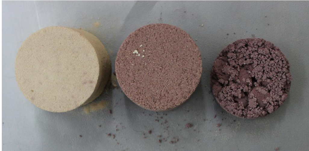
Figure 15 Initial Test Specimens Using Traditional Ramming Method
