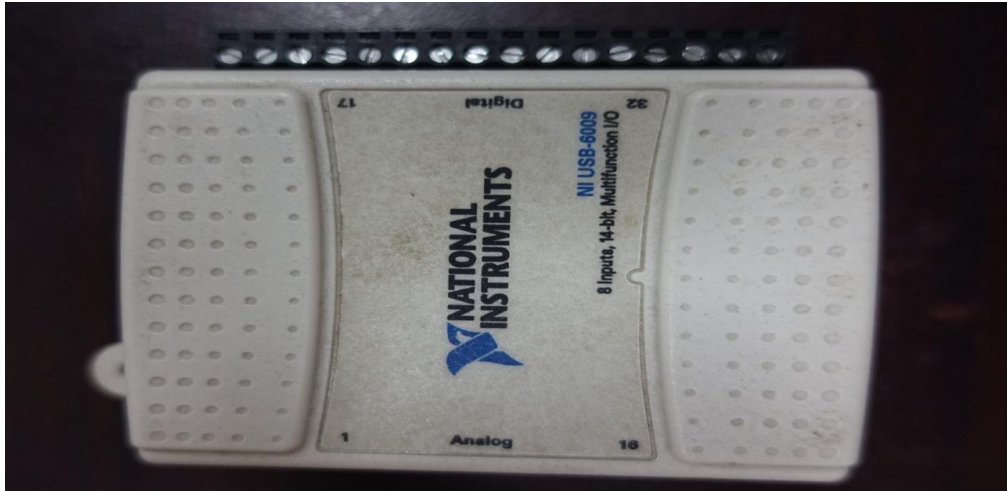
Figure 5-5: Deck Card for attaining analog voltage signal from flapping motion of piezoelectric eel
