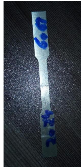
Figure 3.6: Specimen for tensile test
