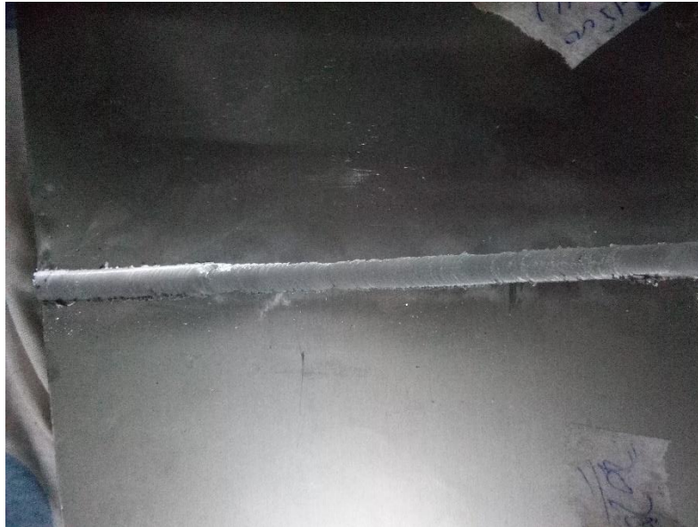
Figure 4.1: Butt joint formed through FSW
