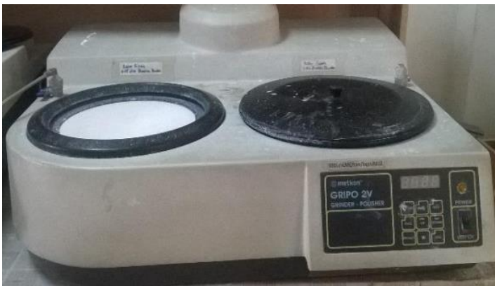
Figure 3.7: Grinding & Polishing Machine
