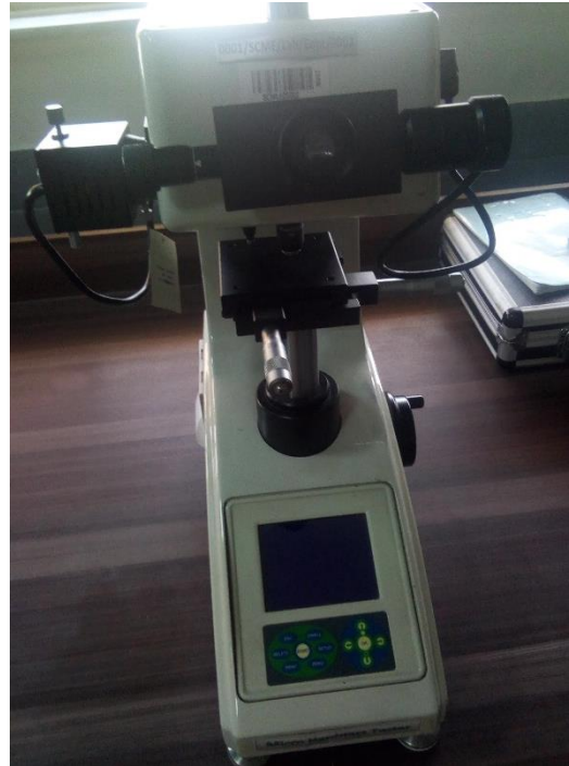
Figure 3.10: Micro-hardness Testing Machine
