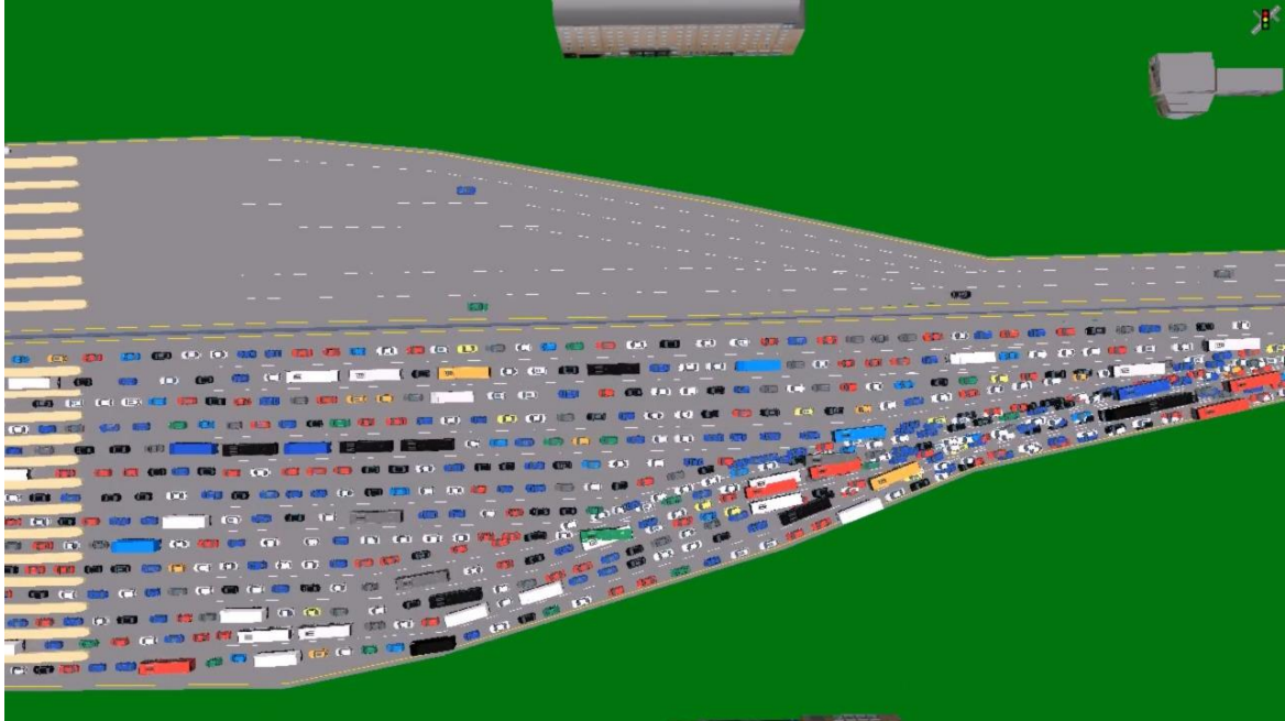
Figure 4. 25 Present infrastructure under traffic conditions after 10 years with 4% traffic growth
