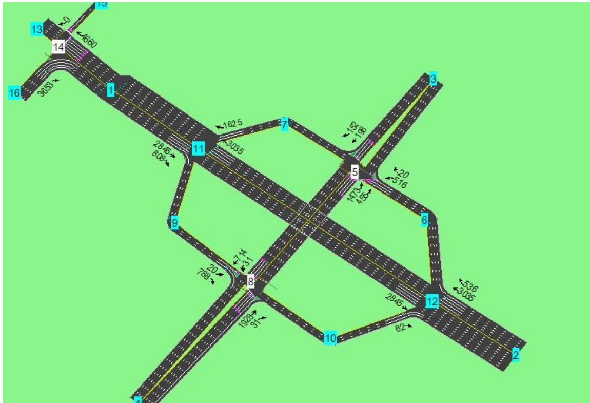
Figure 20: Showing Improved Geometry with Grade Separation
