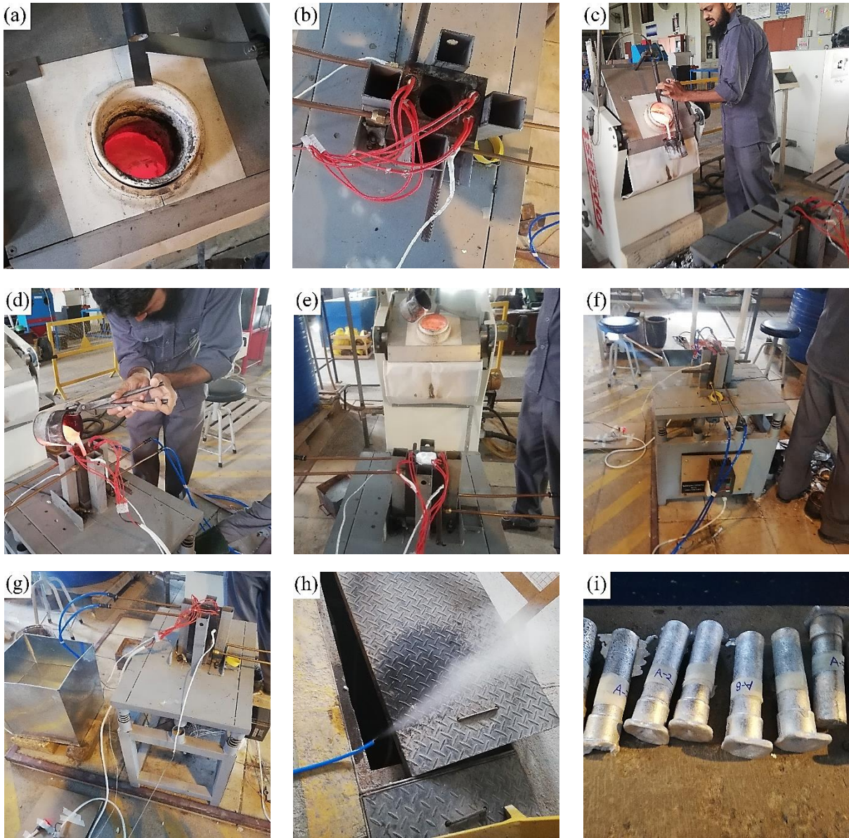
Figure 3-7: (a) Melting in Furnace, (b) Die Pre-Heating, (c) Pouring from Crucible to Pouring Cup, (d) Pouring through Pouring Cup, (e) Vibration On, (f) Vibration Stopped and Holding, (g) Water Pump on for Cooling, (h) Steam Out, (i) Casted Parts
