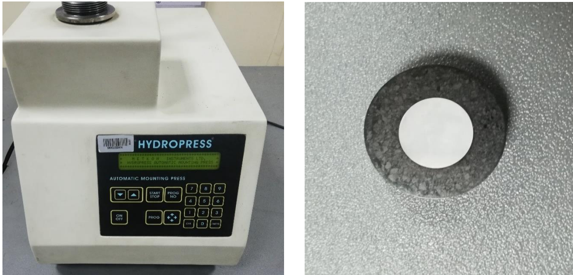
Figure 11: (a) Mounting Machine (b) sample preparation through backlit powder
