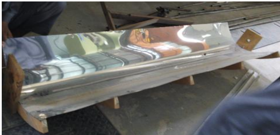
Fig.13 Reflecting sheet with parabola ribs for PTC
