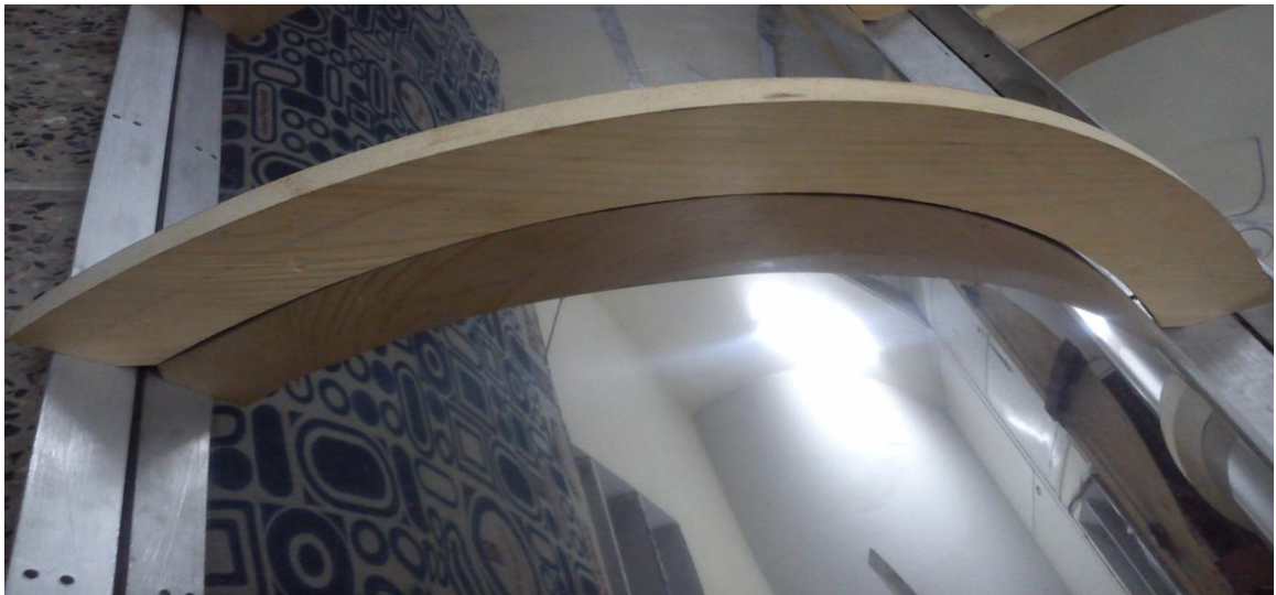
Fig.14 Fixing of side rails with wooden ribs along parabola sheet
