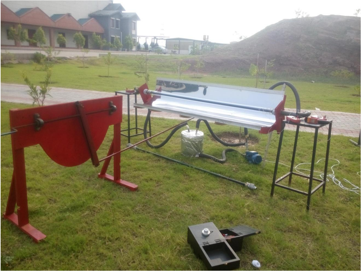
Fig. 29 Experimental Setup of PTC along with Manual Tracing System
