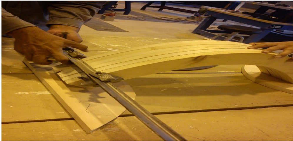
Fig.17 Precise fabrication of wooden ribs for PTC
