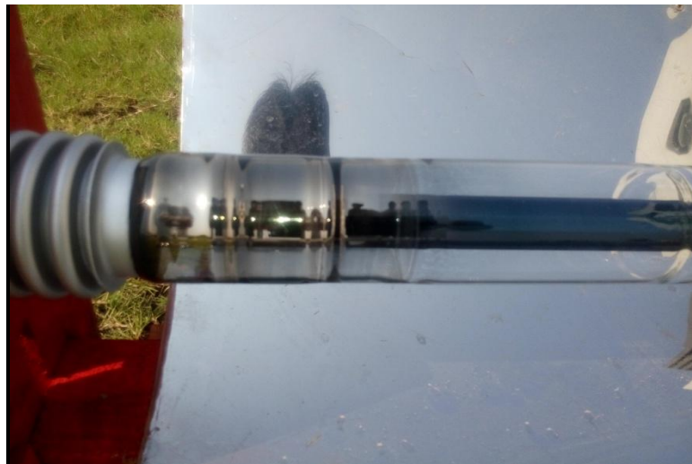
Fig.9c. For Perfect vacuum absorber tubes
