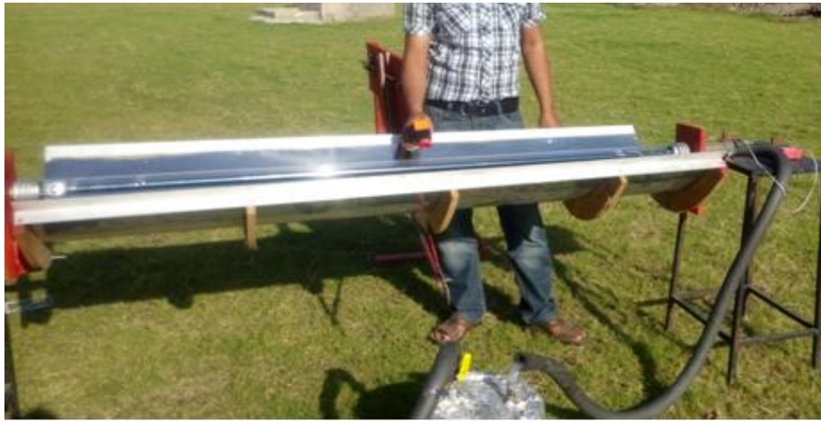
Fig.27 Absorber surface temperature measurement using thermal laser gun
