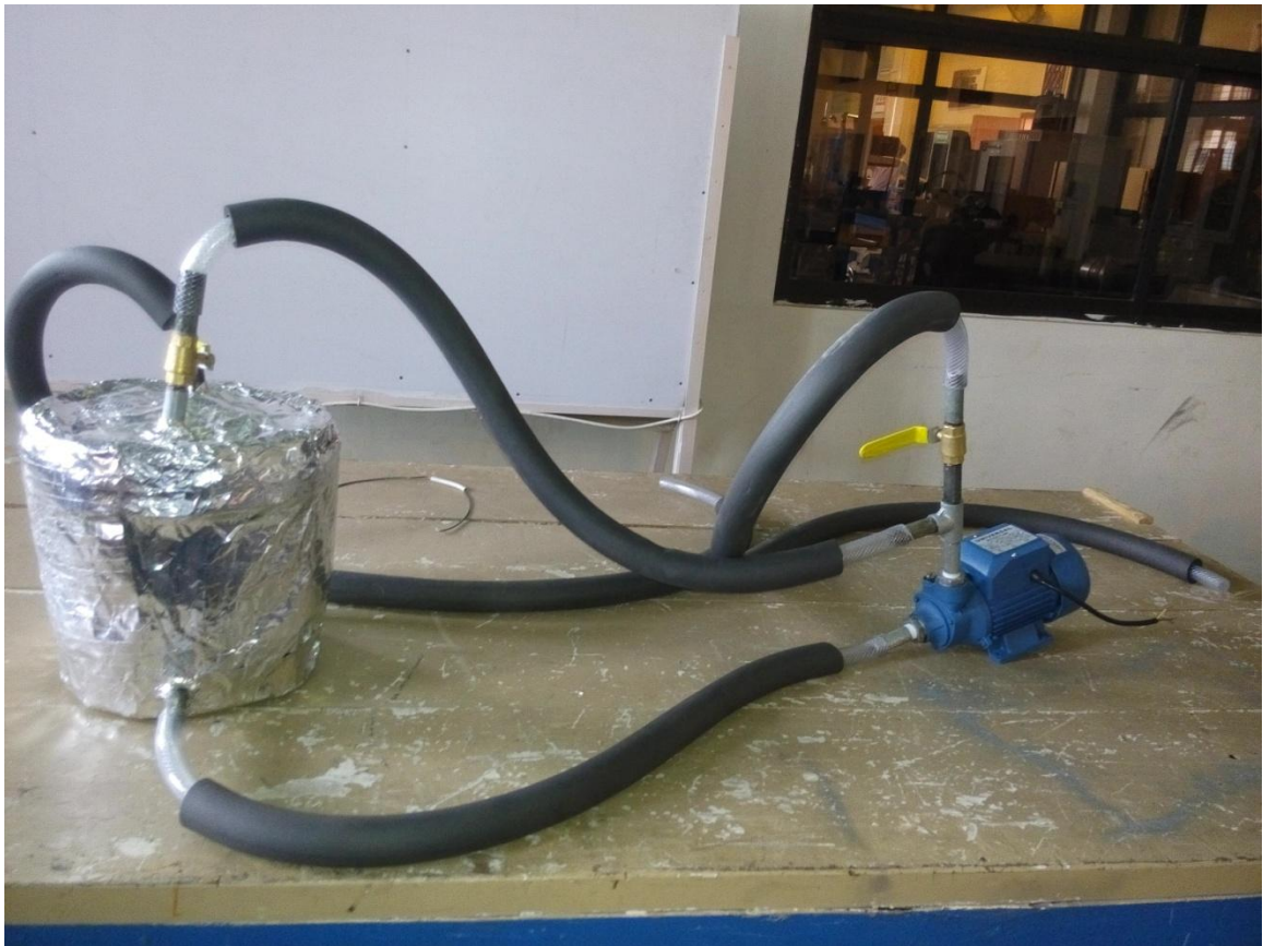
Fig.25 Hydraulic Scheme Used for PTC Experimentation
