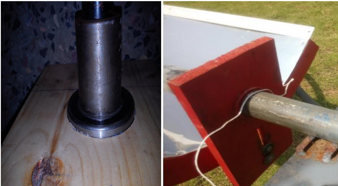
Fig.18 Fixing of bearings in wood
