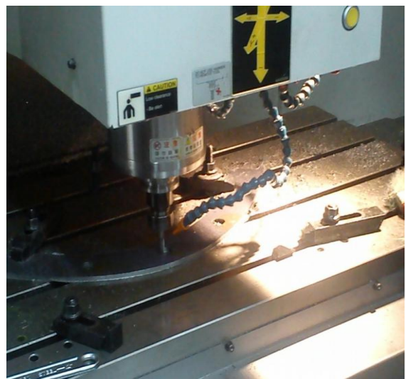
Fig.16 (b) CNC machine used for parabola ribs
