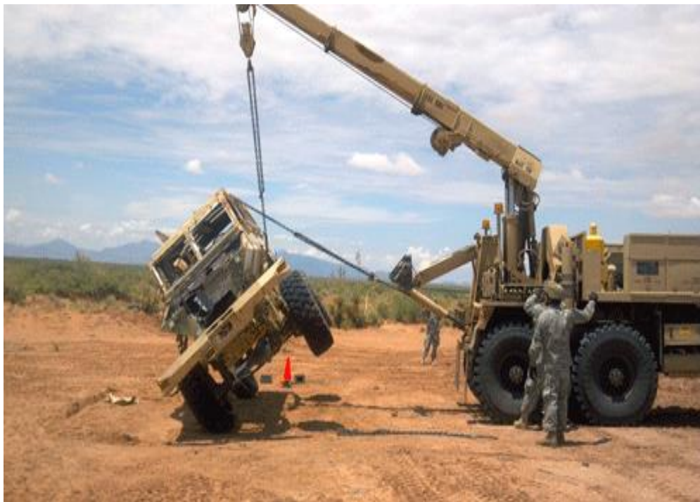
Figure 8 - Mobile Recovery Crane Vehicle
