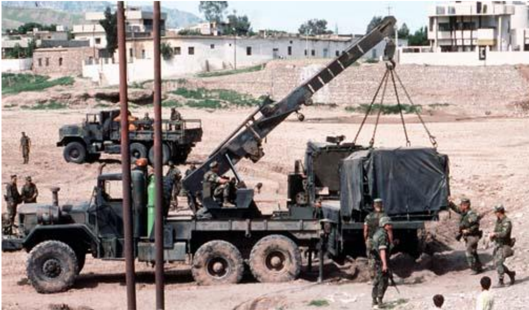
Figure 11 - Recovery Operation in Field Using a Mobile Rotary Crane
