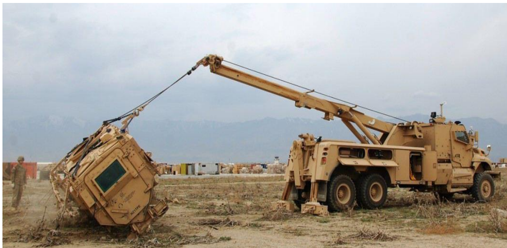
Figure 1 - Recovery Crane Operation in Field
