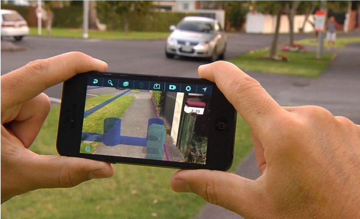
Figure 7 Underground services detection
