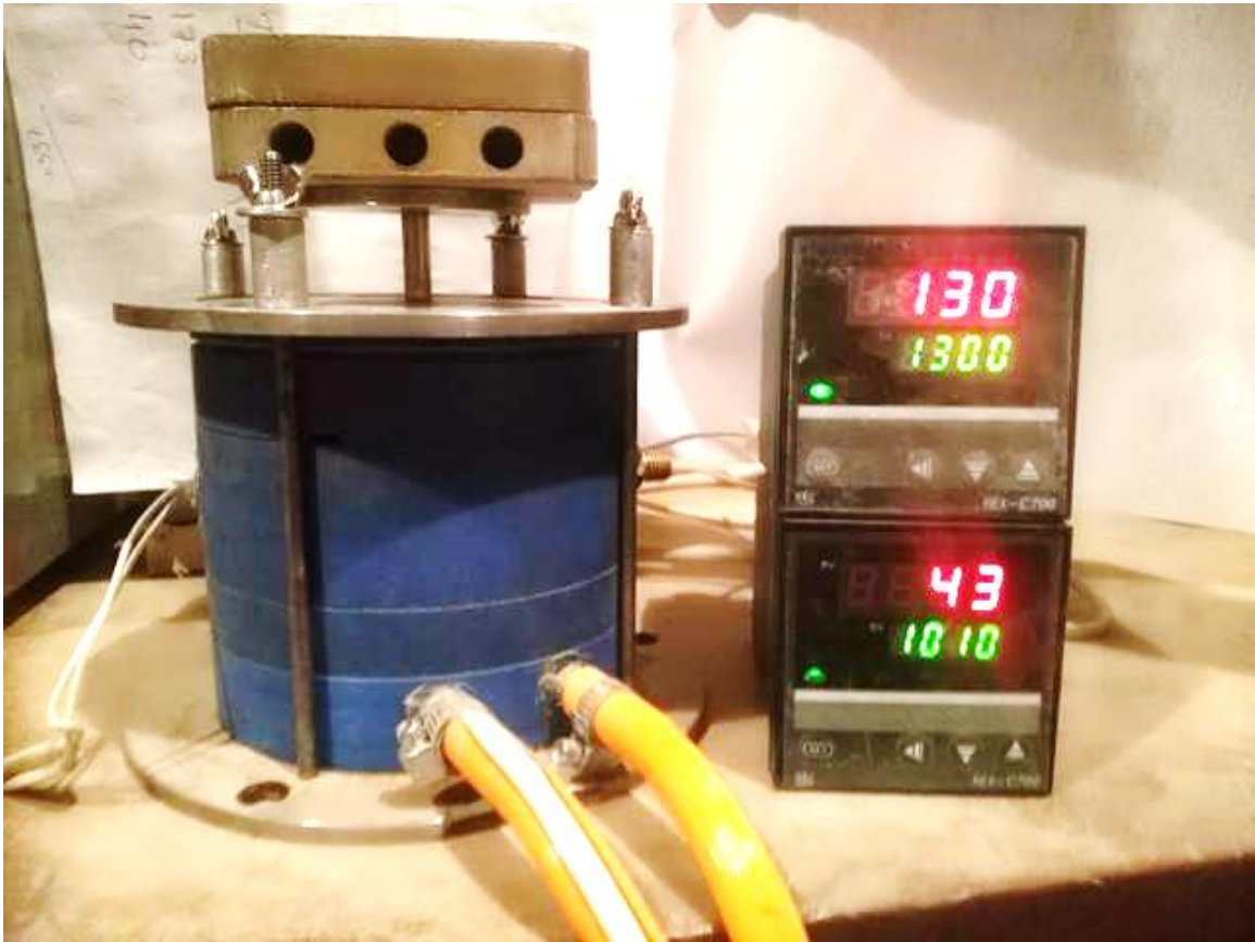
Figure 8. Guarded heat flow meter for thermal conductivity
