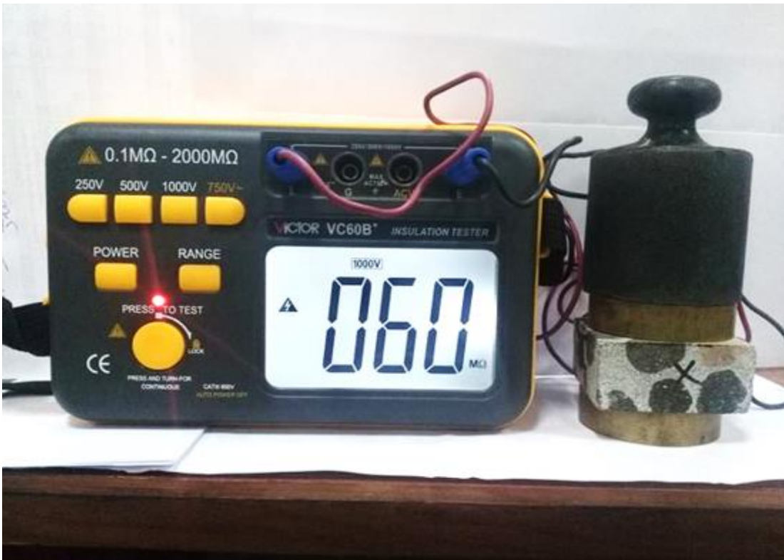
Figure 9. Measurement of Resistivity Using the Two-Electrode Method
