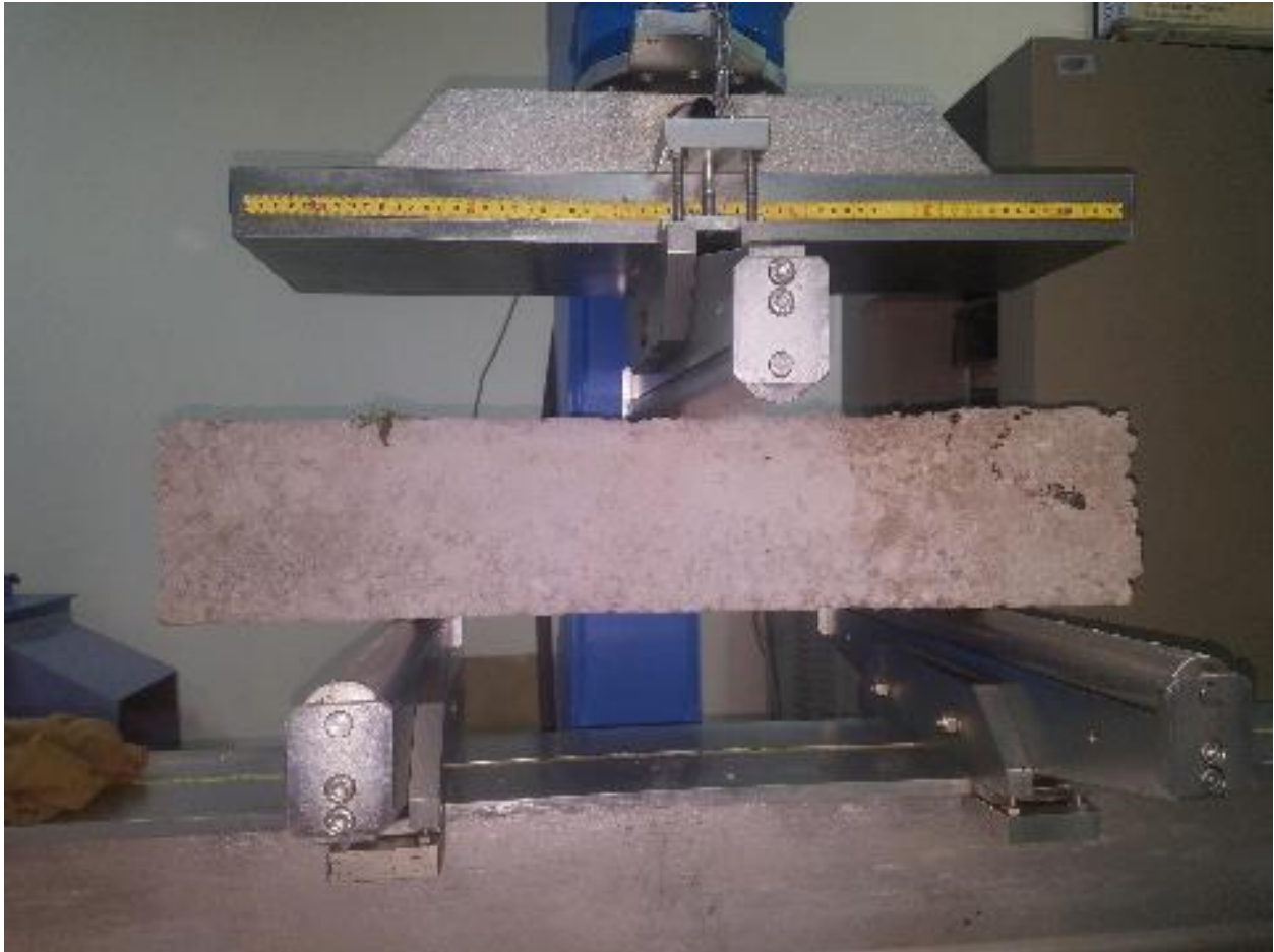
Figure 14: Three point loading test of Hemp rope reinforced beams
