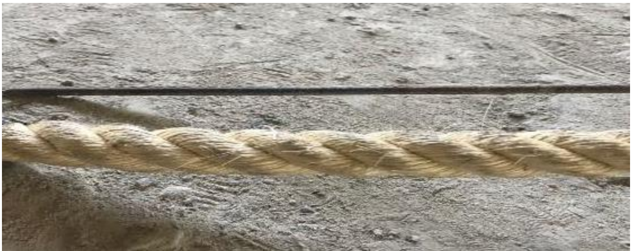
Figure 10: Hemp rope of 1 in. diameter
