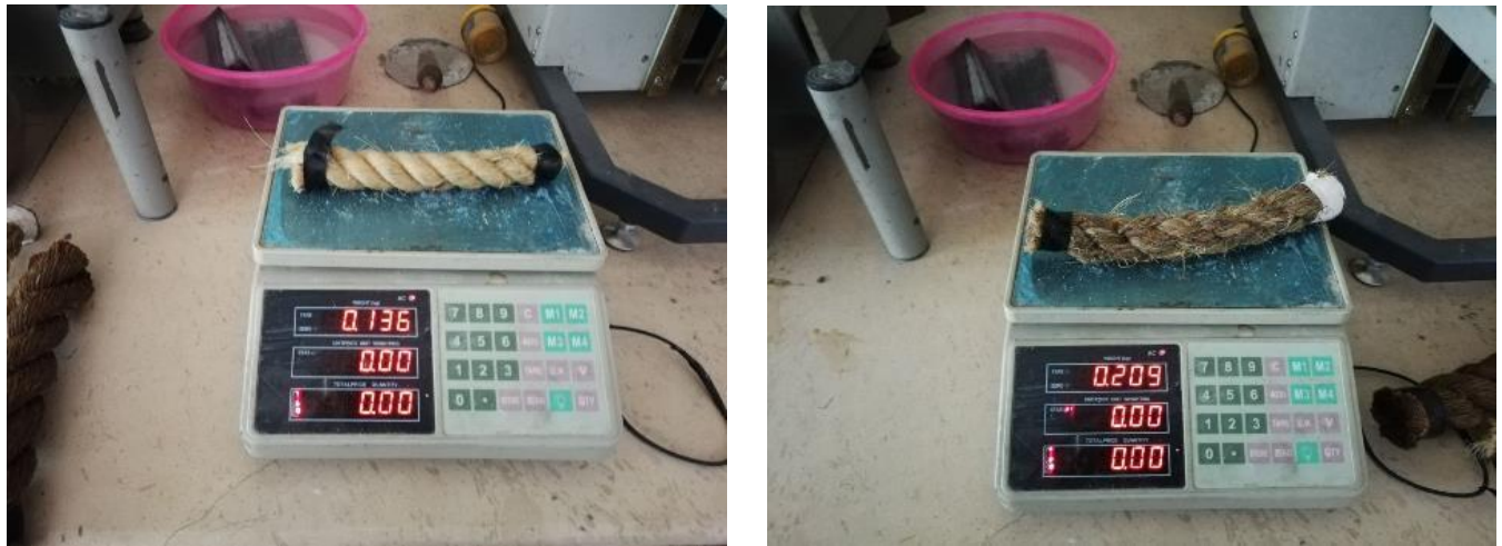
Figure 13: Water absorption tests
