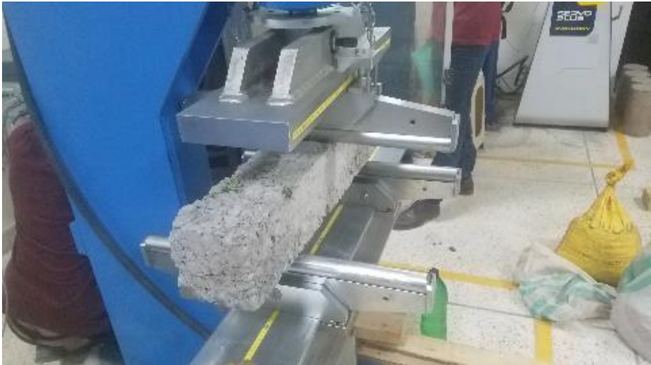
Figure 15: Rope reinforced beam being tested on three point loading testing machine
