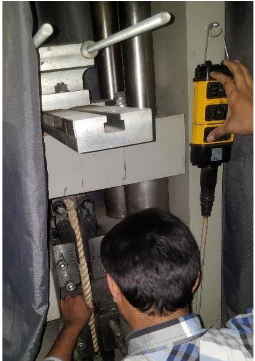
Figure 11: Tensile Strength Test being conducted
