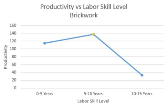
Fig 4.2 Productivity vs Labor skill level (brickwork)
