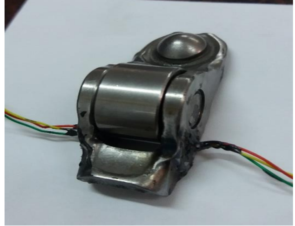
Figure 4.35: Instrumented Toyota Prius Finger Follower
