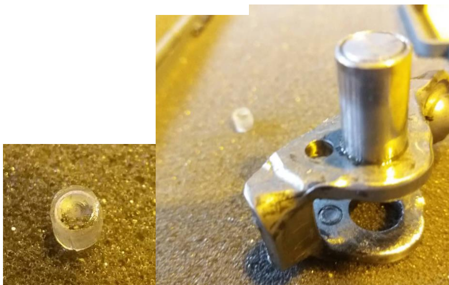
Figure 4.125: Manufactured PCB Holder for Toyota Prius Follower
