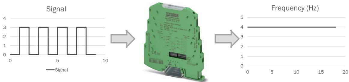
Figure 5.2: Frequency Conditioner Working Principle
