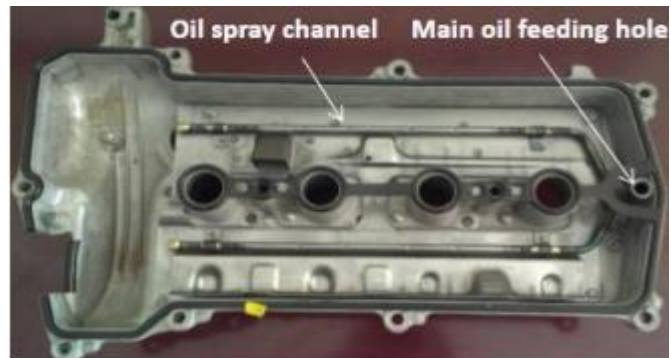
Figure 3.2: Engine head cover having oil spray channel
