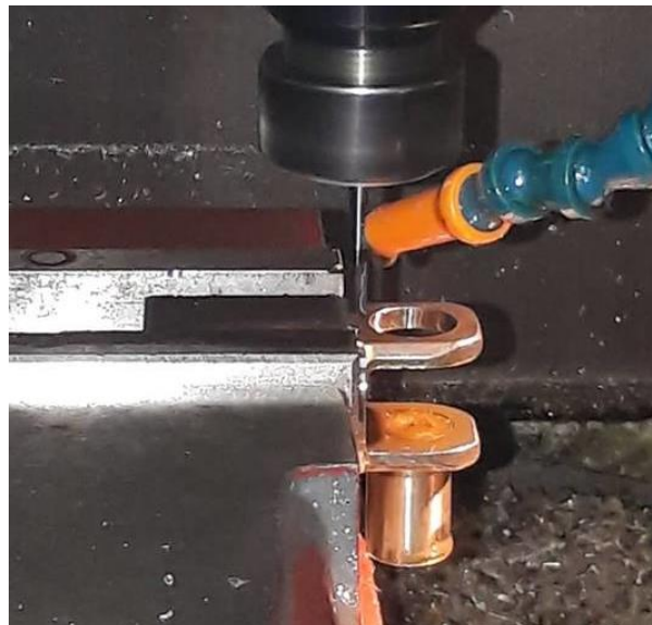
Figure 4.29: Machining of roller casing
