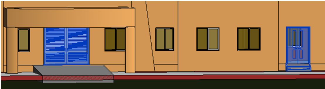
Figure 28 – Non-compliant elements highlighted in BIM model (doors)
