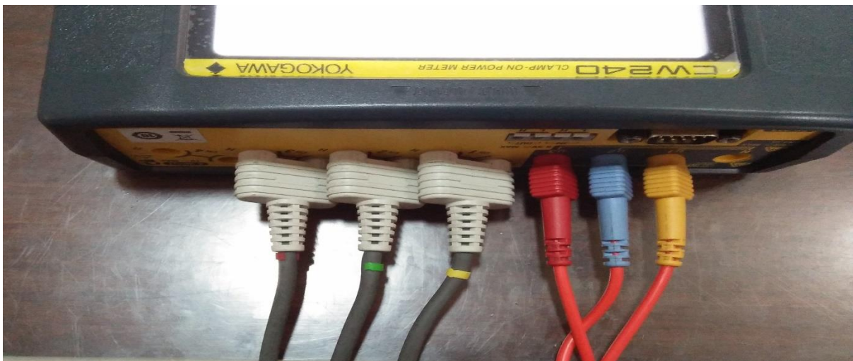
Figure 4.1: Connecting Points of Power Analyzer CW 240-F
