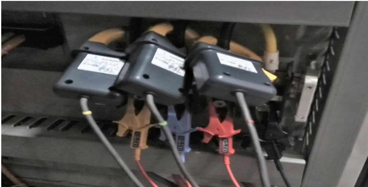
Figure 4.2: Arrangement of Power Analyzer Terminals on Main Bus Bar
