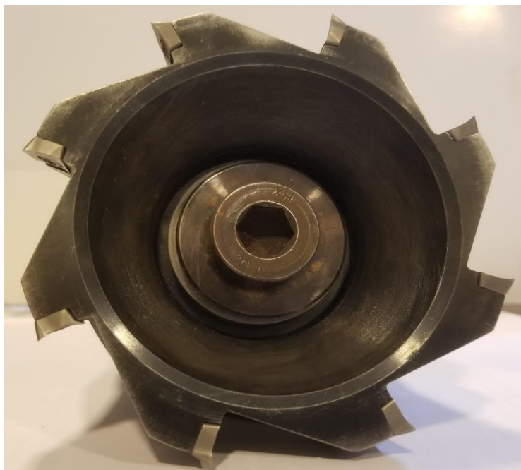
Figure.3.4: Face Shell Milling Cutter Mounted with Uncoated Carbide Inserts
