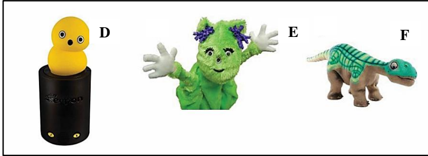
Figure 2.2 Zoomorphic robots Keepon, Charlie and Pleo used in therapies for Autism Spectrum Disorder.
