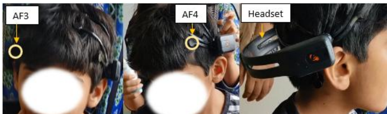
Figure 3.7 Headband adjustment on child's head.
