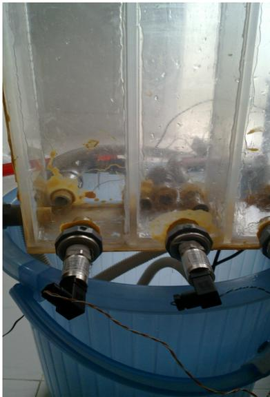
*Figure 4.2: Pressure level transducers attached to the tank.*
