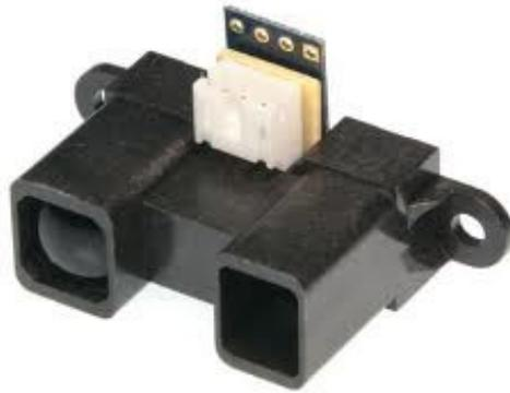
Figure 4.5: Sharp IR (GP2Y0A02YK0F)
