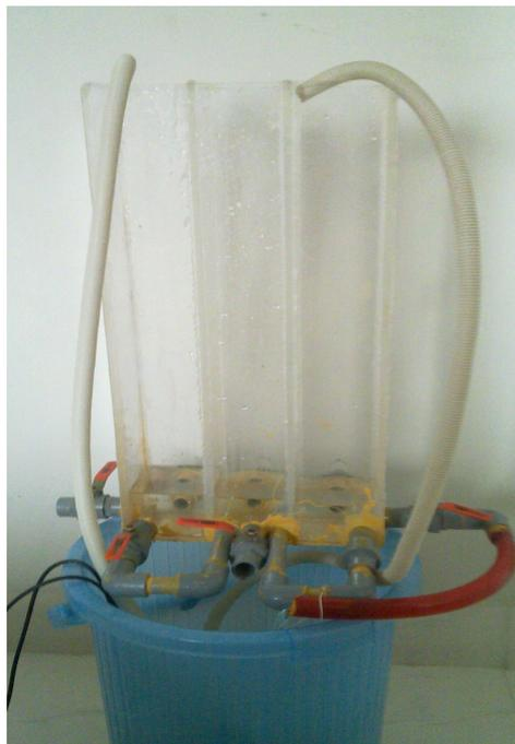
*Figure 4.1: Coupled tank system.*
