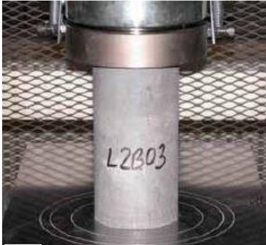
Fig 6. Concrete core testing
