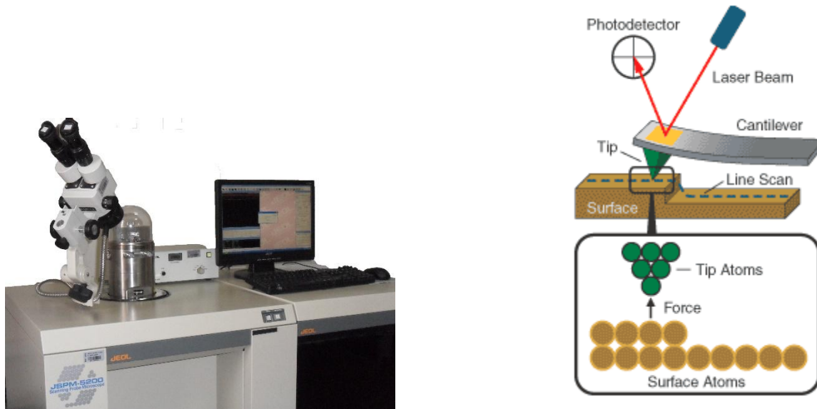
Fig. 3.5. (a) AFM JEOL (JSPM-5200), (b) Schematic diagram of AFM
