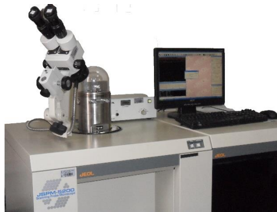
Figure 4-6 JEOL (JSPM-5200) Atomic Force Microscopy (AFM)
