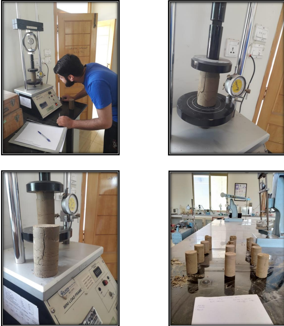
Fig 3.6 UCC test pictorial view
