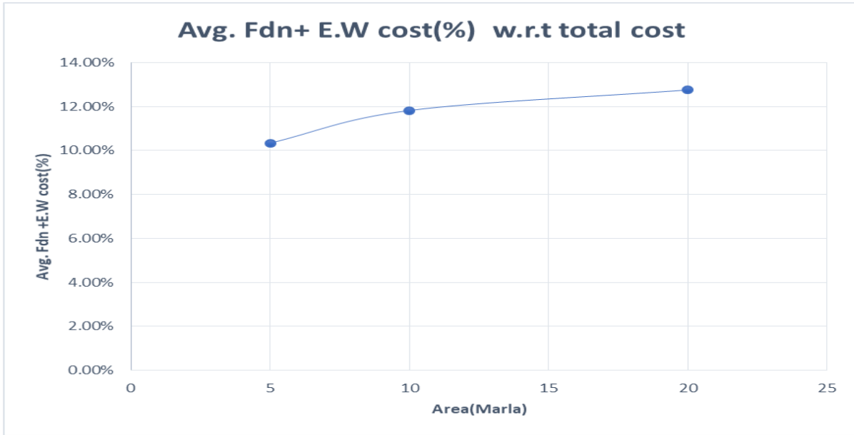
Figure 4-10: Variation of Earthwork + Foundation Proportion with Area
