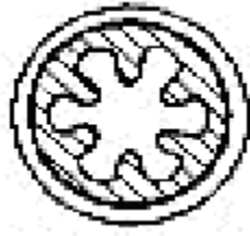
Fig 12 Wagon Wheel Grain Configuration
