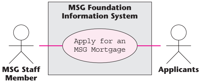
FIGURE 11.5 The Apply for an MSG Mortgage use case of the initial business model of the MSG Foundation case study.
