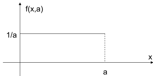
Fig. 2.1. Probability density function of a random variable X , uniformly distributed on the interval [0, a]
