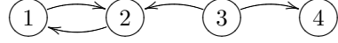
Fig. 1.3 The set C = \{1, 2\} is a final class, State 3 forms a passage class by itself and State 4 is absorbing.
