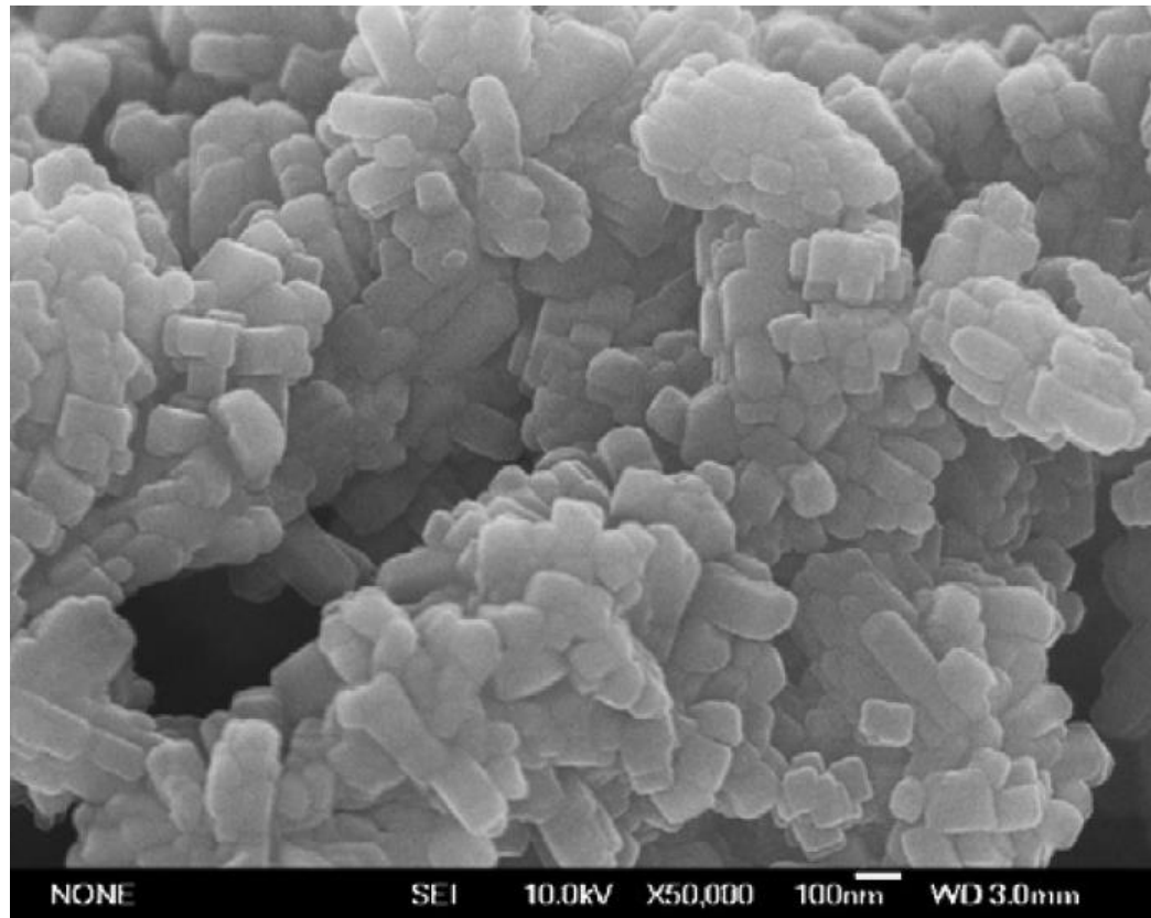
Figure 3.9 SEM for Nano CAT (Bi, 2009 )
