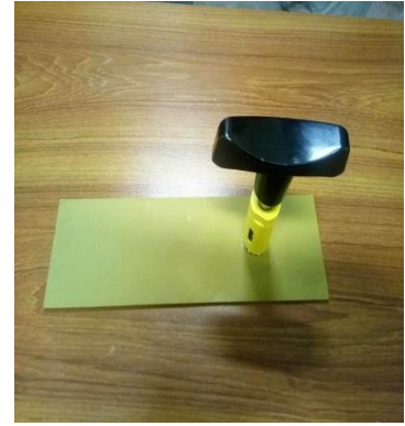
Figure 4.16 Puller attached to the dolly
