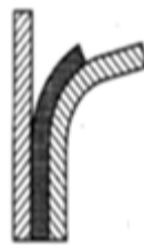
Figure 2.2: Adhesion failure of adhesive [90]
