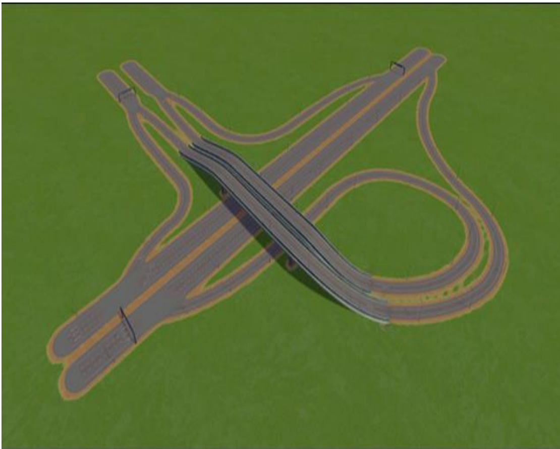
Figure 4 Image showing a Trumpet Interchange
