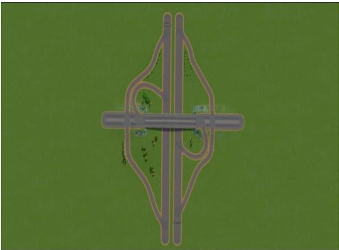
Figure 7 Image showing Partial cloverleaf interchange
