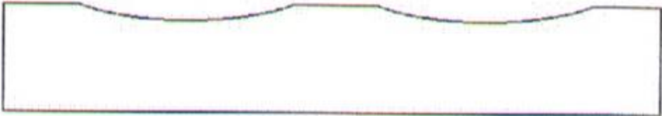
Figure 2-2 Consolidation-Depression along the wheel path.
