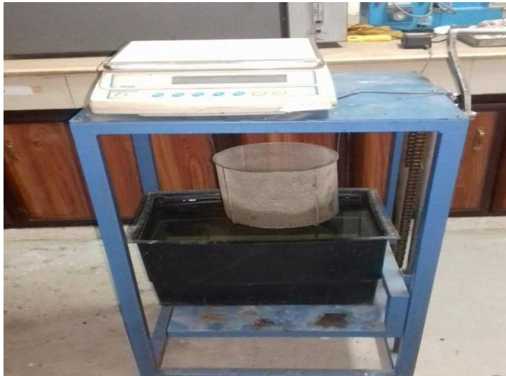
Figure 3.10. Gmb Calculation for Marshall Samples.
