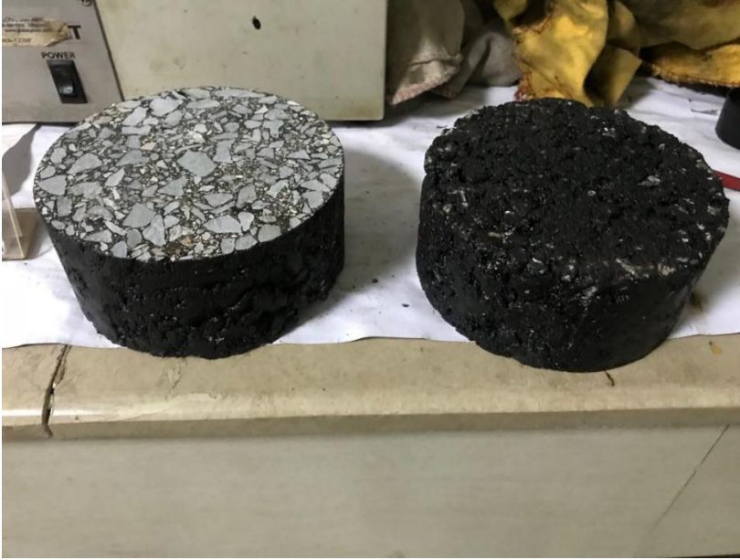
Figure 3.11 Sample Cut with Help of Saw
