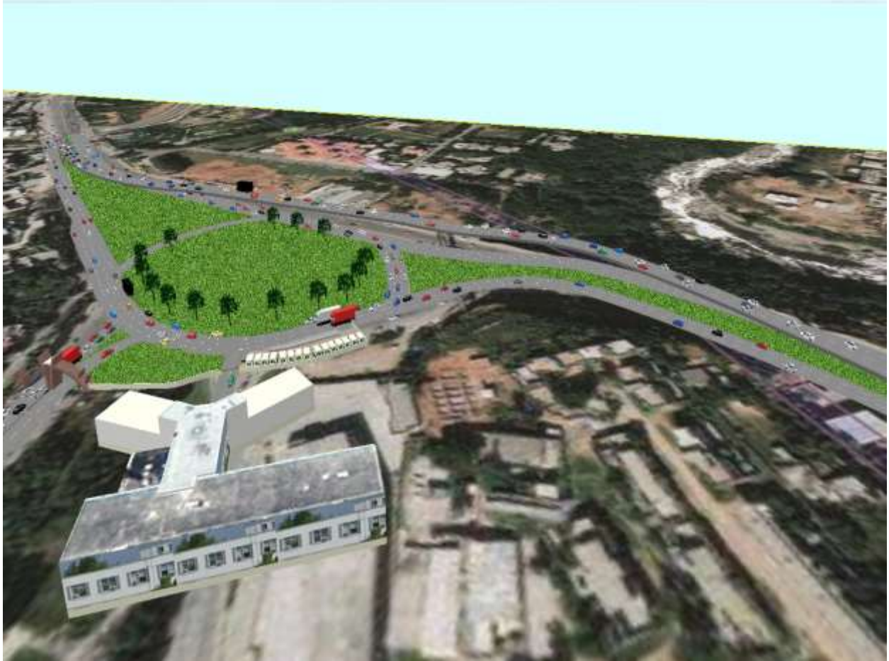
PTV VISSIM generated model of Defence Roundabout
