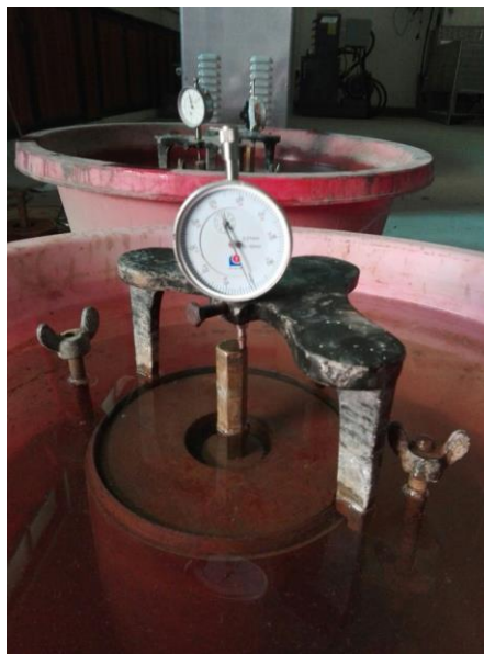
Figure 3.7 Soaked CBR Mould
