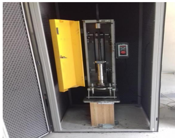
Figure 3. 16: :Compaction of Sample
